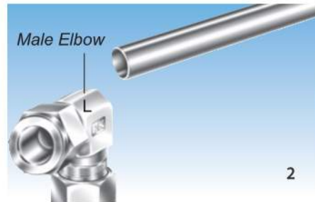
The male elbow is positioning in the wrong direction.
